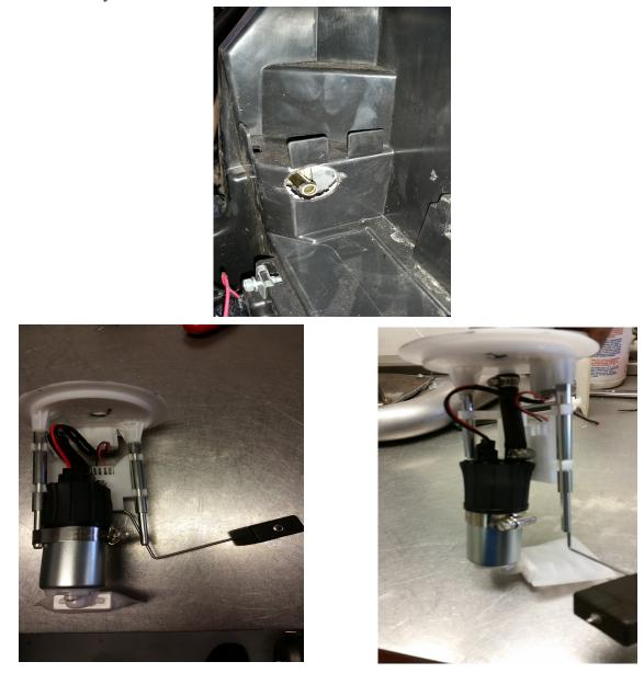
Remove the stock fuel pump from tank. Remove the pump from assembly and install the supply pump with hose, clamps and solder wires to plug as shown above. With supplied fuel pump temp plate drill 1/2 hole in top plate for return fitting seen in picture.
