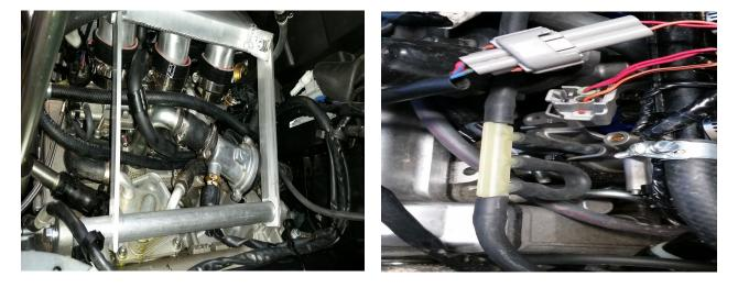
Install intercooler support kit as shown in picture below. Install 3 supplied intercooler couplers on throttle bodies and clamp tight. Remove rubber cap from rear vacuum nipple on rear throttle body and push on the short 7/64 vacuum hose from manifold kit as picture shows. Connect one vacuum hose to Hurricane control box and let the other hose hang behind engine.
