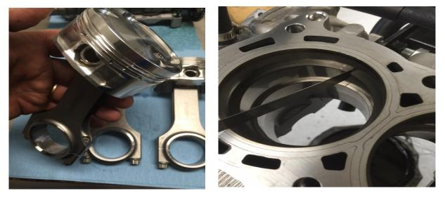
Rings are installed on pistons and ready for cylinders. Notice the shinny molly ring is the top ring and marking is up. Place the ring gaps 45deg's apart on piston. Oil piston rings before re-installing pistons into block.
