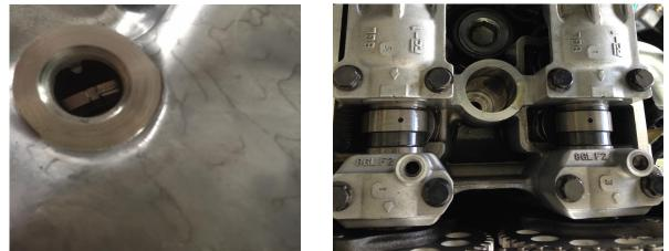
The Yamaha torque spec is 10nm. We torque them to 9nm because an aged engine often will pull the threads at 10nm
