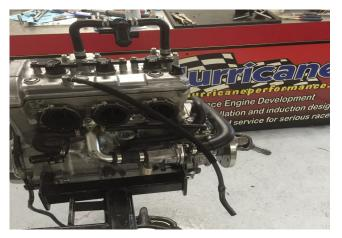
Re-gap the spark plugs to .018in. Reinstall valve cover, coils, coolant and air hoses. Remove factory plug on head at rear of throttle bodies and install supplied oil supply fitting with brass washer..... Be careful not to over-tighten. Before reinstalling your motor your need to prepare your fuel system. As shown in picture use a step drill bit. To drill 1/2 hole inside centre console to allow fuel return hose from the regulator to follow stock fuel line layout.
