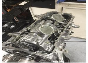
Clean the stud with brake clean and apply red loctight to the threads as they enter the block. Screw 7 of the studs to the bottom. **Do not tighten**. The 8<sup>th</sup> stud at the water pump apply lots of lock tight and install at **depth of 82mm** from deck level. Let the lock tight cure before torquing the head at water pump.
