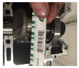
After bearings clearance you need to lubed both of rods bearings and re-torqued 45lbs. Be sure to align the balance shaft to crank as below. The hole with pink paint on crank lines with the hole mark on the balance shaft. Yamaha Bond along the outer part of lower case and reinstall using the stock torquing. specifications.
