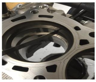
Rings are installed on pistons and ready for cylinders. Notice the shinny molly ring is the top ring and marking is up. Place the ring gaps 45deg's apart on piston. Oil piston rings before re-installing pistons into block.
