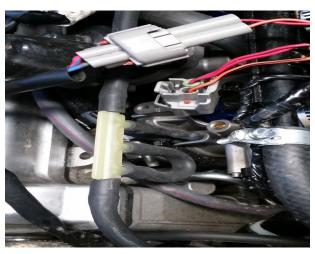
Install intercooler support kit as shown in picture below. Install 3 supplied intercooler couplers on throttle bodies and clamp tight. Remove rubber cap from rear vacuum nipple on rear throttle body and push on the short 7/64 vacuum hose from manifold kit as picture shows. Connect one vacuum hose to Hurricane control box and let the other hose hang behind engine.
