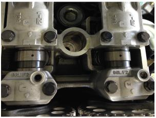
The Yamaha torque spec is 10nm. We torque them to 9nm because an aged engine often will pull the threads at 10nm
