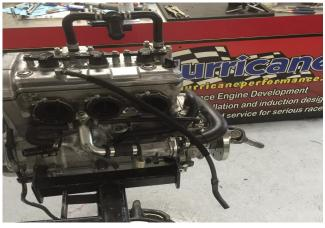
. Reinstall valve cover, coils, coolant and air hoses. Remove factory plug on head at rear of throttle bodies and install supplied oil supply fitting with brass washer.....
