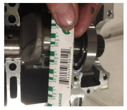
After bearings clearance you need to lubed both of rods bearings and re-torqued 45lbs. Be sure to align the balance shaft to crank as below. The hole with pink paint on crank lines with the hole mark on the balance shaft. Yamaha Bond along the outer part of lower case and reinstall using the stock torquing.
