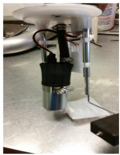
Remove the stock fuel pump from tank. Remove the pump from assembly and install the supply pump with hose, clamps and solder wires to plug as shown above. With supplied fuel pump temp plate drill 1/2 hole in top plate for return fitting seen in picture.
