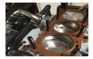
Install the ARP washers first. Lube the nuts with Carrillo bolt lube or equivalent. Torque the head down in **three steps** from the centre outward starting at **35lb** torque, then **45lb** then **55lb**
