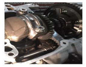
Install the oil pump making sure your drive chain is on the crank shaft out drive and oil pan installed.
