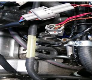
Install intercooler support kit as shown in picture below. Install 3 supplied intercooler couplers on throttle bodies and clamp tight. Remove rubber cap from rear vacuum nipple on rear throttle body and push on the short 7/64 vacuum hose from manifold kit as picture shows. Connect one vacuum hose to Hurricane control box and let the other hose hang behind engine.
