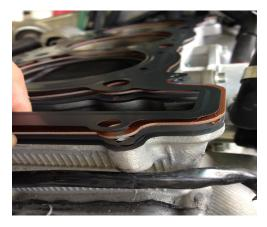
Install the ARP washers first. Lube the nuts with Carrillo bolt lube or equivalent. Torque the head down in **three steps** from the centre outward starting at **35lb** torque, then **45lb** then **55lb**
