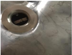
Clean the stud with brake clean and apply red loctight to the threads as they enter the block. Screw 7 of the studs to the bottom. **Do not tighten**. The 8<sup>th</sup> stud at the water pump apply lots of lock tight and install at **depth of 82mm** from deck level. Let the lock tight cure before torquing the head at water pump.
