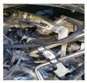
Lay Hurricane control box over centre console. Connect injector connectors to stock injector plugs and injectors with wire colours matching injectors at firewall Green, middle Yellow, rear injector Orange. Plug in TPS and crank sensor connectors and ground Hurricane control box. Connect the supplied jumper cable to stock air temp connector and lay across the motor.
