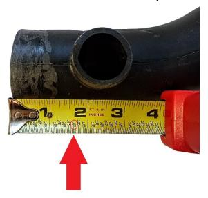
3) Sand the casting imperfections off the pipe from the new edge to about the nipple. This should allow a tight fit to work the Hurricane Turbo 998 Intake Adaptor to index it for proper clearance to the steering shaft and alignment with the turbo inlet
