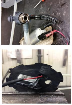
Drill 1/2in hole in stock sending unit for fuel return and install supplied fitting and grommet as shown in picture and template suppled.
