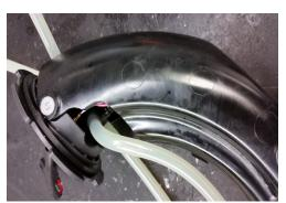
Remove factory fuel pump from tank. As showen in picture below. Remove both white plastic clips and remove fuel bowl from pump assembly.
