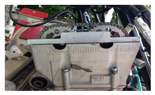
Rotate engine in running direction to set chain tension and re-align timing marks as shown in timing picture. Loosen cam gear bolts and install cam timing jig as shown in picture. Be sure that the flat part of bolt hex rests on jig. Apply red loctight librally to cam gear bolts and tighten with wrench.
