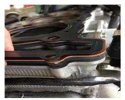
Lower head down over studs and install supplied washers. Lube nuts with molly style lube and torque from center outwards. Torque specs are first stage (35lbs),second stage(45lbs),third stage(55lbs) using a well calibrated torque wrench.
