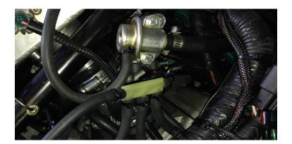
Remove factory plug from end of the fuel rail. Remove rubber O ring from plug and install it on new regulator. Install the supplied fuel regulator to rail. Connect the fuel return line from the tank to the regulator. Cut part of the blow off valve hose supplied and connect the hose from intercooler nipple to the fuel regulator.
