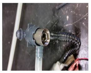
At this piont remove the black fuel hose and screen filter from factory pump. Connect fuel hose and screen filter to supplied in-tank pump. Plug in pwer and ground wires to pump. Re-install the fuel pump back into fuel bowl.
