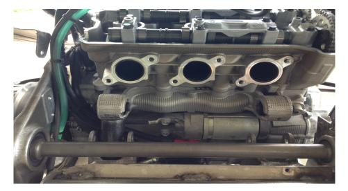
Remove valve cover and heat exchanger vent tube after motor is raised. This will allow chain tensioner to be removed after the timming marks are aligned as picture below.
