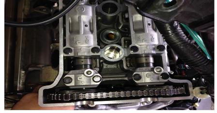
Remove cam chain tensioner, cam caps and cams. Remove head bolts and cylinder head. DO NOT TIP HEAD UPSIDE DOWN TO ALLOW VALVE BUCKETS TO FALL. Clean block and head surfaces with acidtone. Clean threads in block and ARP studs with brake clean. Apply red loctight on studs that enter the block. Set left front head Stud depth to 82mm above block deck as shown in picture. Then install the other 7 studs into block with red loctight till they bottom.
