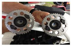
Slot bolt holes in cam gears and reinstall on cams.
