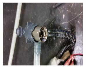
Drill 1/2in hole in stock sending unit for fuel return and install supplied fitting and grommet as shown in picture and template suppled.
