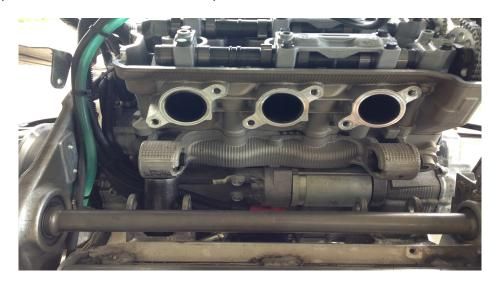
Remove valve cover and heat exchanger vent tube after motor is raised. This will allow chain tensioner to be removed after the timming marks are aligned as picture below.
