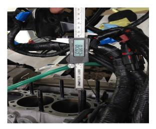
Split the supplied head gasket by pulling it apart. Spray copper coat to each side of supplied stainless head shim. Install one half of head gasket over studs followed by shim and finaly other half of head gasket as picture shows below.
