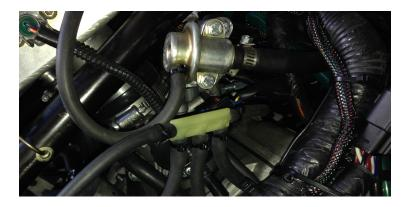
Remove factory plug from end of the fuel rail. Install the supplied fuel regulator to rail. Connect the fuel return line from the tank to the regulator. Cut part of the blow off valve hose supplied and connect the hose from intercooler nipple to the fuel regulator.
