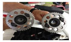
Install cams in head and set dot alignment to caps as shown in previous timing picture. Install chain tensioner with the word UP to top.
