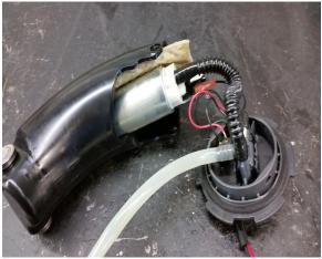
Re install fuel pump sysyem back into tank. Re-connect fuel line and add your return fuel line with gromet suppled in kit.
