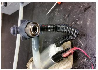
While holding on to the regulator and using a T-handle 6mm to tighten the screw all the way in till it bottoms out as per picture on the right.
