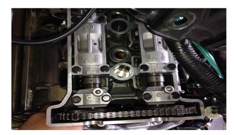
Remove cam chain tensioner,cam caps and cams. Remove head bolts and cylinder head. **DO NOT TIP HEAD UPSIDE DOWN TO ALLOW VALVE BUCKETS TO FALL**. Clean block and head surfaces with acidtone. Clean threads in block and ARP studs with brake clean. Apply red loctight on studs that enter the block. Set left front head Stud depth to 82mm above block deck as shown in picture. Then install the other 7 studs into block with red loctight till they bottom.
