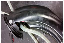
Remove factory fuel pump from tank. As showen in picture below. Remove both white plastic clips and remove fuel bowl from pump assembly.
