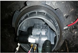
Unclip black plastic clip from regulator. Pull out factory regulator held in by rubber groumet from plastic housing.
