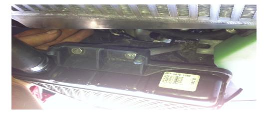
Install the 2 supplied radiator support bolts and bushings as shown in the picture.
