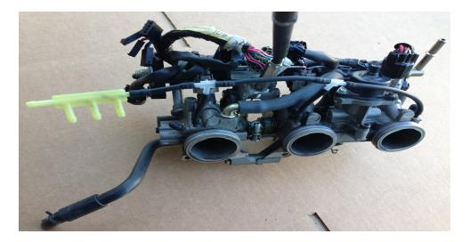
Install the oil return fitting into the stator cover. Remove screw beside throttle bodies on the head and install oil supply fitting with copper gasket from screw. (**Do not over tighten fitting**)
